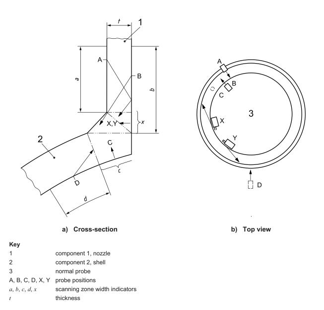
Figure A.5 —Set-on nozzle joints
